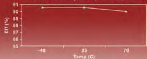
DC500S-28 Efficiency vs Temp at Io=20A, Vin=28V
