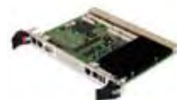
CR11 6U Compact PCI single board computer with Intel® Core™2 Duo or Intel® Core™ Duo processors
